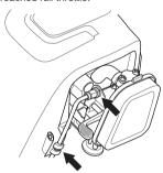
Adjust the nut on the throttle cable with the nut. Then tighten the lock nut.
