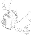
Once engine is started leave the choke lever in Half choke position for 20 seconds. Then move the choke lever to RUN position.
